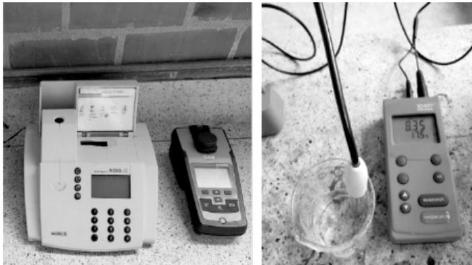
Figure 7. Colorimeter, turbidimeter and pH meter.
