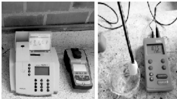
Figure 7. Colorimeter, turbidimeter and pH meter.
